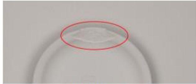
(a) Deterioration after pressing.
