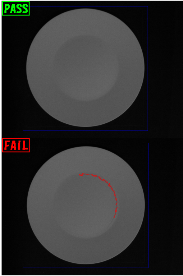
Fig. 4. Evaluation of plates surface defects. Top image: Passed inspection for surface defects. Bottom image: Failed inspection for surface defects.
