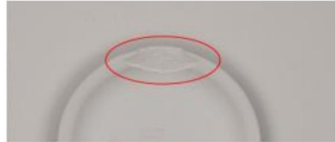
(a) Deterioration after pressing.
