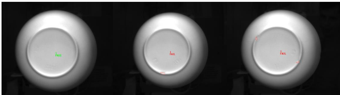
Figure 3: Detecting cracks on the back of the plates. Left image: Passed inspection. Middle and right images: Failed inspection.
