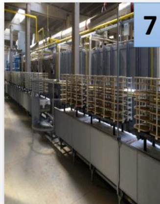
Biscuits dipped into glaze mixtures (matte or glossy, containing various concentrations of pigments)
