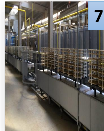
6 Biscuits dipped into glaze mixtures (matte or glossy, containing various concentrations of pigments)
